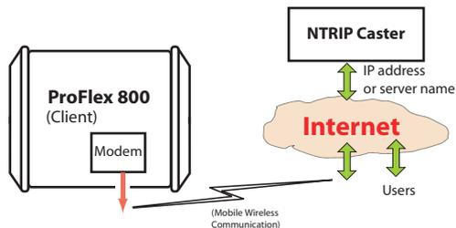
The internal modem should be configured first:
