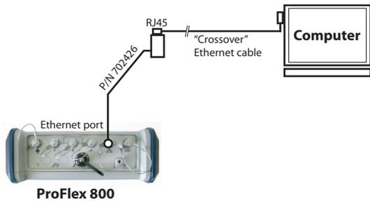
This type of connection is required when the receiver is not otherwise using its Ethernet port and there is no network connection available in the operating environment of the receiver (machine control, machine guidance).
