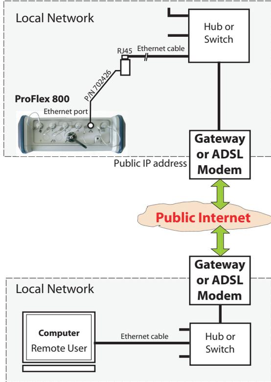
In this configuration, the IT Manager should take all the necessary steps for users to be able to access the ProFlex 800 through the public IP address of the local network. **Obviously, the IP address read on the receiver display screen is NOT the one to be provided to users.**
