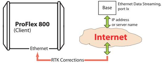
The rover needs to be configured as in Direct IP mode via Ethernet (see *Direct IP Via Ethernet on page 22*).
